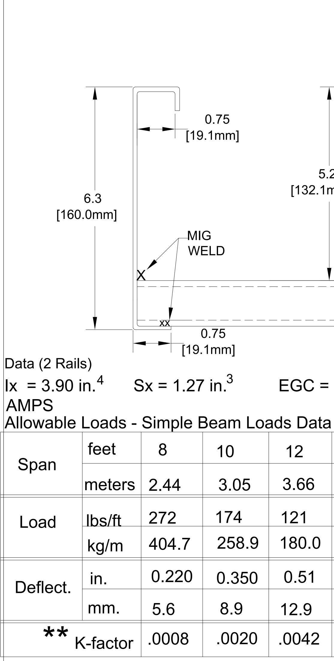
\*\* K x W may be used to calculate deflection of lighter loads at indicated space above
