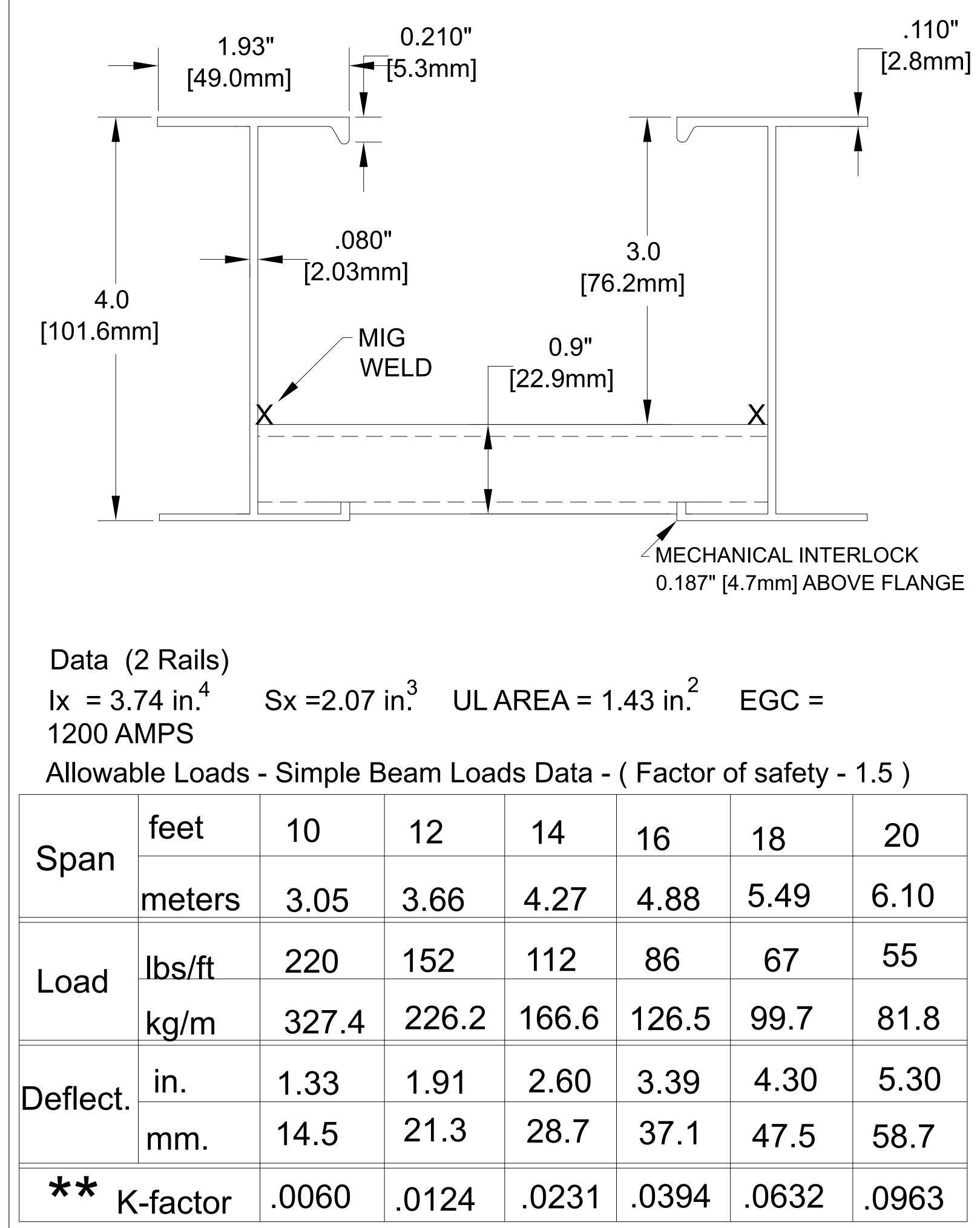
\*\* K x W may be used to calculate deflection of lighter loads at indicated space above
