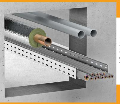
If cables are run through building walls or ceilings, then the fire resistance must be restored with cable insulation. if, in addition, different installations such as electrical cables or sanitary pipes run through the same opening, then combination insulation is used.
