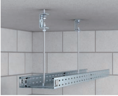
Installation of center suspension Installation of the central suspension MAH 60 on the ceiling using threaded rod 2078/M10 and ceiling bracket 12050. Maximum cable trough width 12\".
