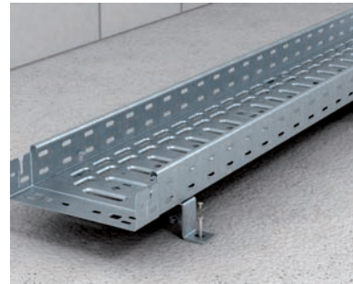
Floor fastening at a distance Installation of a cable trough at a distance using the stand-off bracket DBL. Maximum cable trough width 24\".
