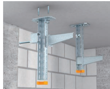
Standard mounting of support with wall and support bracket, single-sided with spacer Cover fixing of a suspended support with single-sided bracket fixing. For widths of over 16", we recommend using a spacer.
