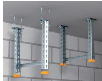
Traverse Installation of U suspended supports US 3 K, US 5 K and US 7 K under the ceiling using anchor bolts and use as a trapeze, consisting of U profile US 3, US 5 or US 7.
