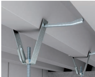
Installation of trapeze suspension Installation of a cable trough on a trapezoidal ceiling using a ceiling bracket, type TPB 100 and central suspension, type MAH 60. Maximum cable trough width 12". The trapezoidal fastening is mounted using the lock, type TPB R.
