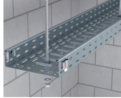
Center suspension with threaded rod Direct center suspension at low loads of a cable trough with threaded rod 2078/M10.
