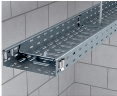
Installation of central suspension MAH 60 Insertion and alignment of the central suspension, MAH 60, in the cable trough.
