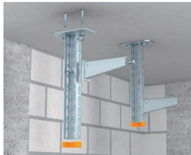
Standard mounting of suspended support with wall bracket, single-sided without spacer Cover fixing of a suspended support with single-sided bracket fixing. No spacer is required for widths up to and including 12".
