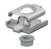
Screwed version of joint connector for mesh cable trays. Figure: Positioning and quantity of mesh cable tray connectors. 50-150 mm = 2 units 400 mm = 3 units 450-600 mm = 5 units Including FRS M6 x 20 bolt with flange nut.
