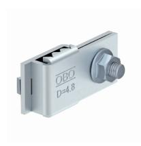
The connection and earthing terminal is used to reduce electrical resistance and therefore improves the electric conductivity in mesh cable systems in the area of the joint allowing to fulfil the high demands in terms of the transition resistance according to e.g. NEMA and CSA. Furthermore, the connection and earthing terminal is compulsary when used as a protective conductor in a mesh cable tray system (Note: National regulations have to be followed when creating such a system).
