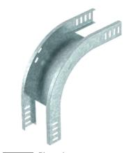
The vertical bend is pushed over the end of the cable tray and screwed tight. Fastening materials should be ordered separately.  $90^{\circ}$  vertical bend, falling, for all cable tray types of 35 mm side height.
