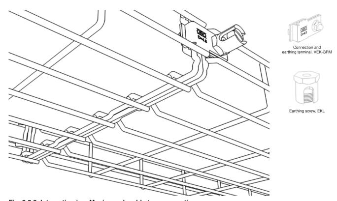
Fig. 3.5.2. Integration in a Magic mesh cable tray connection
