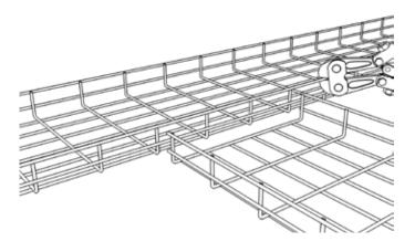
**Fig. 4.2**Notching out of the side grids on both mesh cable trays to be con-
