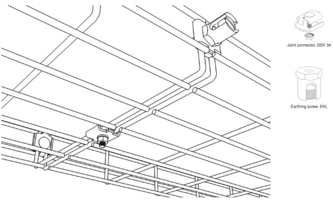
Fig. 3.5.1 Integration of a cut mesh cable tray
